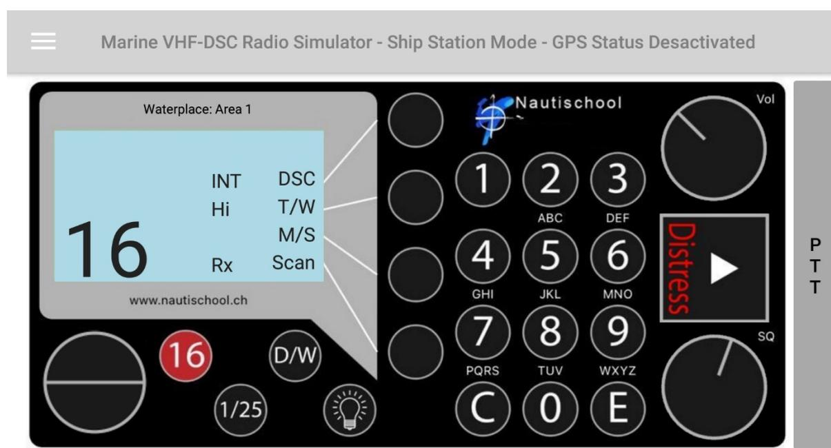
Turn the rotary control (1) to begin and adjust the squelch (2)
