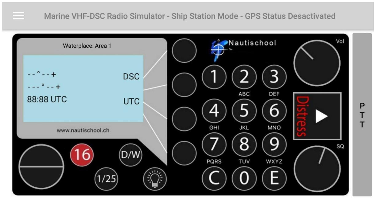
4. Enter Latitude and Longitude using keypad and N, S, E, W softkeys when available
