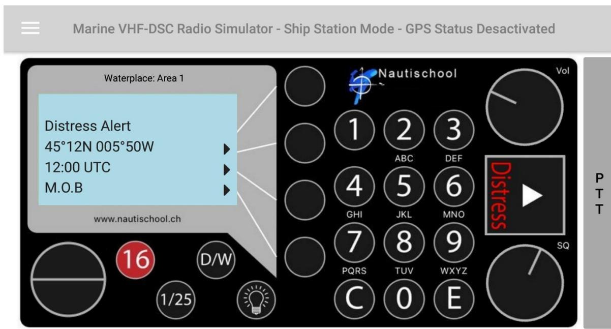
Press and hold the DISTRESS key for 5 seconds. A countdown to the transmission will be displayed. Release the key at any time during this countdown to abort the transmission.
