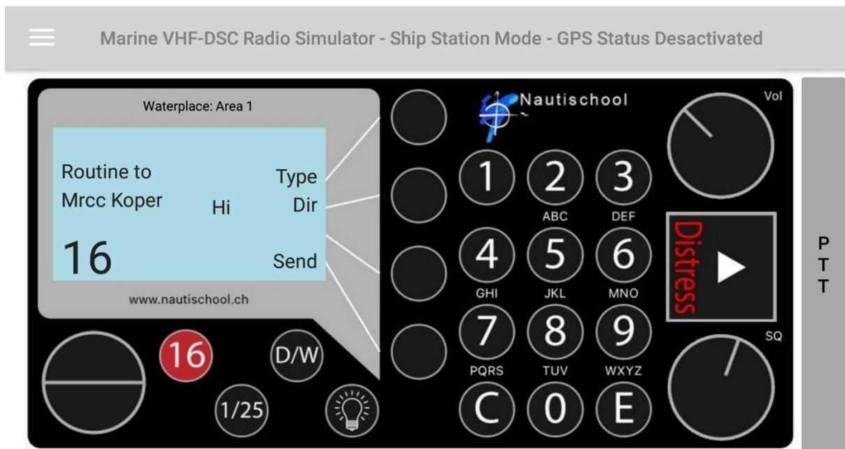
By default, MrccKoper is shown. It's a costal station, you can directly send an alert to MrccKoper and wait for an acknowledgment on channel 16 by pressing Send and E.
